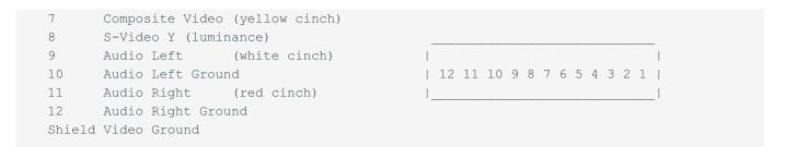
The standard AV-cable connects only to Pins 7,9,10,11,12,Shield (with pin 1 and 3 and Shield shortcut with each other, used for both audio and video ground).
